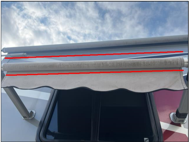
Residue on Awning
