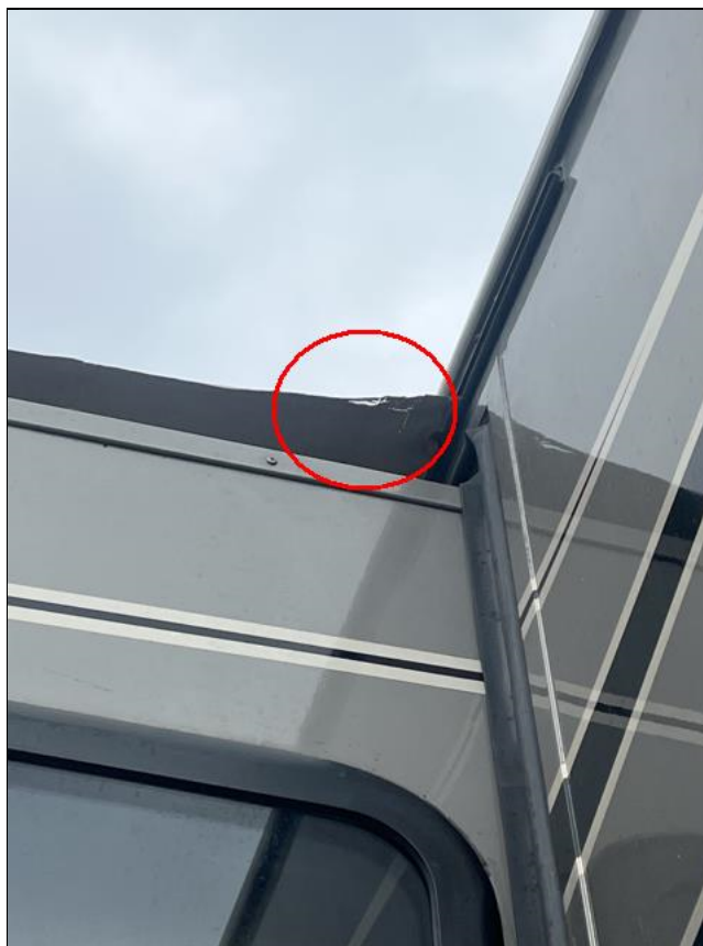
Damaged Awning Material
